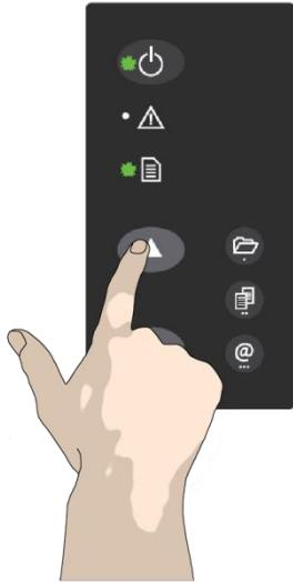
press and hold down the Paper Forward button on the scanner.
