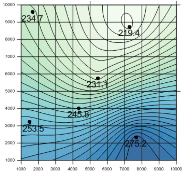
*The irregularly spaced data points are used to interpolate grid node values. These interpolated values are written to a grid file. The grid file is used to produce the contour map. This figure shows the filled contour map, the posted data points, and the layout of the grid.*
