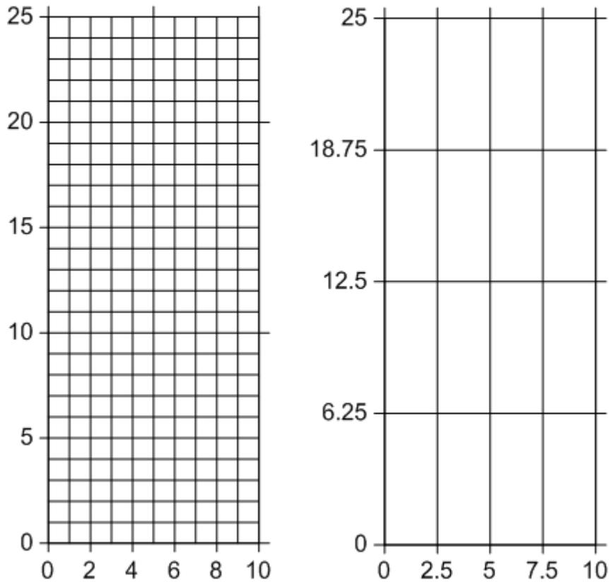
*Two different Grid Line Geometry examples are shown here. These are based on the same data file. The coordinates range from zero to 10 in the X direction and zero to 25 in the Y dimension.*
