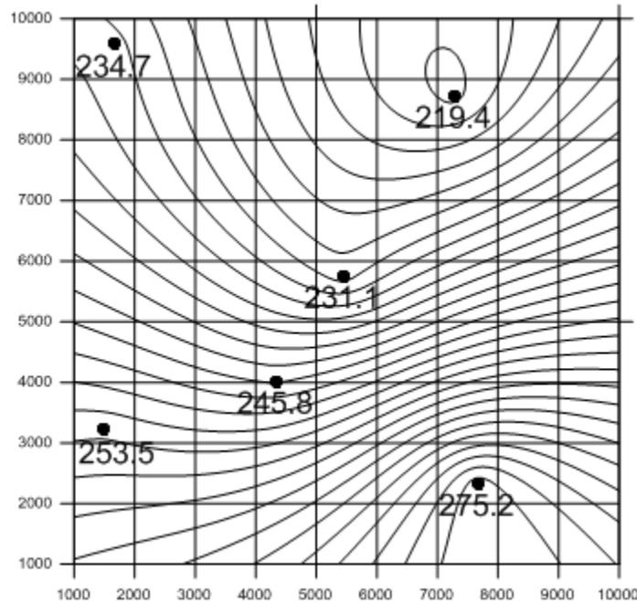
*The post map layer shows the original data points. The contour map layer shows the grid based contour map.*
