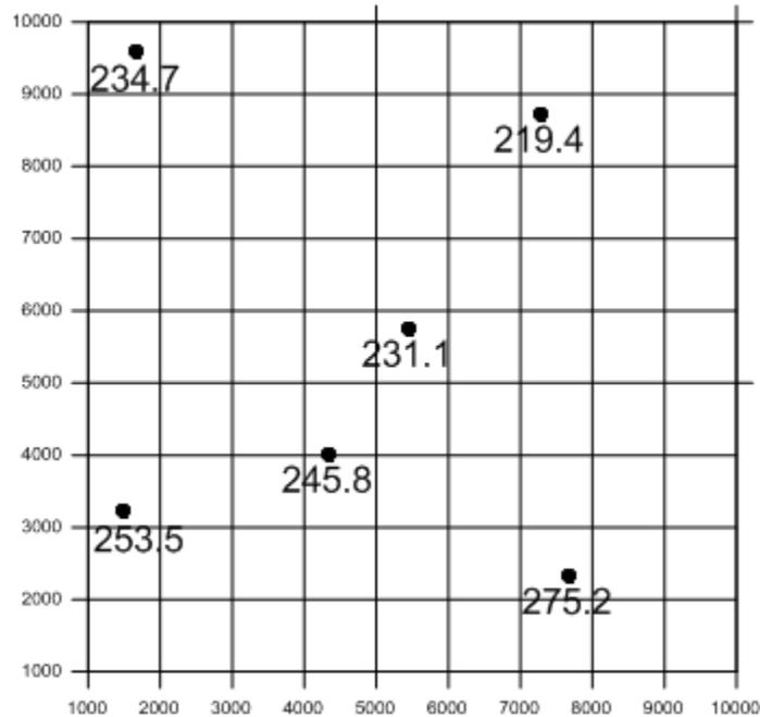
*Gridding interpolates a Z value at the intersection of each row and column in the grid file, thereby filling holes in the data. Here the rows and columns are represented by grid lines drawn across the map.*
