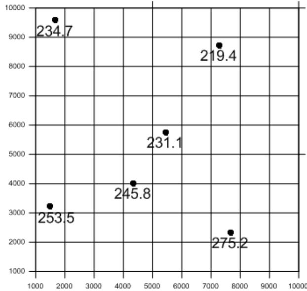
*Gridding interpolates a Z value at the intersection of each row and column in the grid file. This fills the holes in the data. Here the rows and columns are represented by grid lines.*
