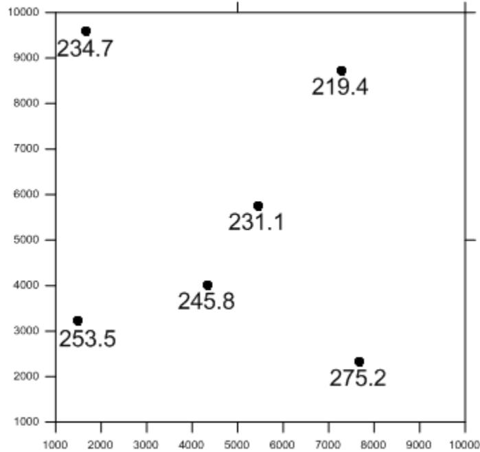
*This is a post map displaying the data locations. The well locations are irregularly spaced over the map in this example. There are many "holes" where no data exists.*
