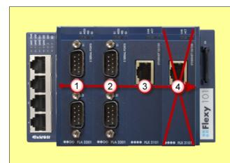
Example of configuration that would be OK mechanically and power wise, but that is not supported by the firmware.
