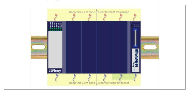
**Caution:** In any other mounting position than the one explained here above, the specified temperature has to be derated to -25°C to +40°C.
