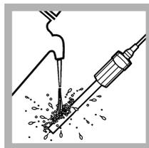
**4.** Rinse the probe with deionized water. Blot dry with a lint-free cloth.
