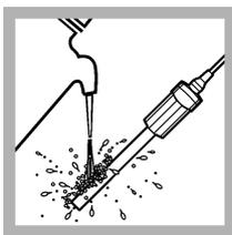
3. Rinse the probe with deionized water and then with the sample. Blot dry with a lint-free cloth.
