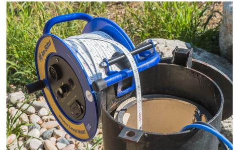
2. Using the sensitivity dial, turn on the meter and adjust to the desired sensitivity.
